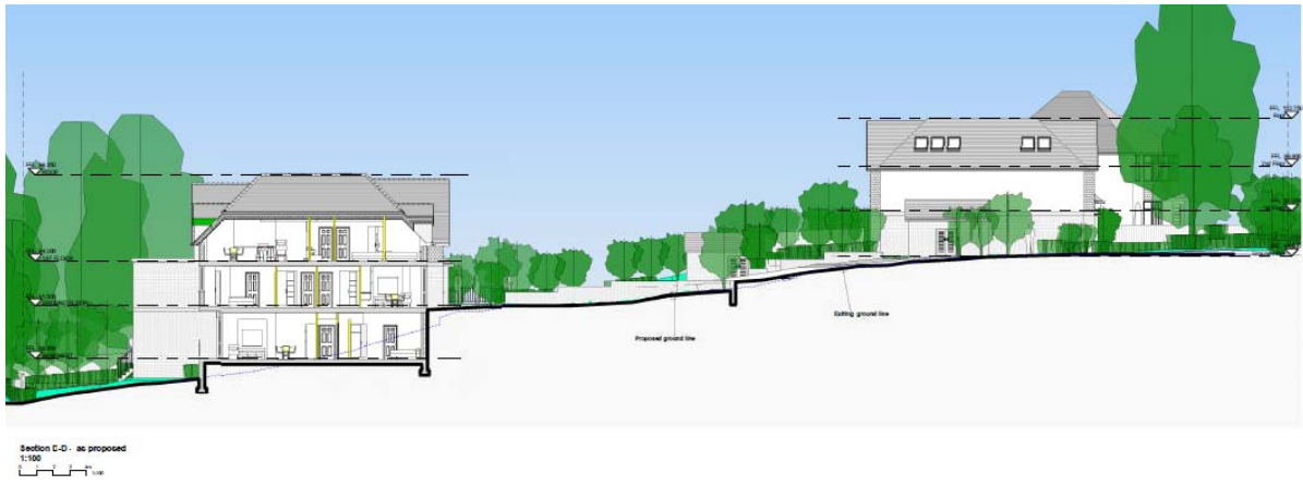
Figure 1 Site cross section showing front block on right hand side is higher than rear block which follows the land levels of the site
